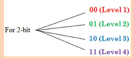
**Quantizing** 0.4 V sample value: See that level 2 is near to 0.4 V. So, for sample voltage 0.4 V, 01 code is transmitted.
