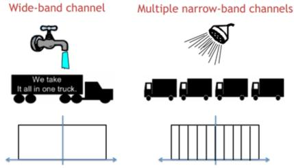
Here in above figure, four smaller trucks represent four sub-carriers in OFDM system and these sub-carriers must be orthogonal to each other. In case of FDM (wide-band channel) data will be transported using entire bandwidth. In OFDM multiple narrow-bands are used and each carry part of data stream.
