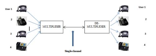
FDM extends the concept of single carrier modulation by using multiple sub-carriers within the same single channel. The total data rate to be sent in the channel is divided between the various sub-carriers. Note that the data neither have to be divided evenly among sub-carriers, nor from the same information source. Each chunk of data can use different modulation technique.
