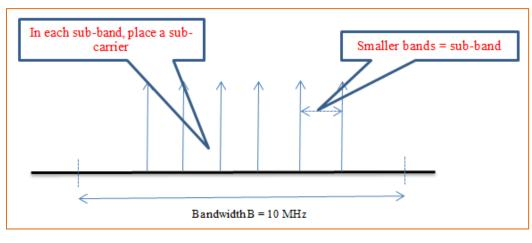
Let B = Bandwidth of channel = 10 MHz N = Number of sub-carriers or sub-bands = 1000 Bandwidth of each channel = B/N = 10 MHz/1000= 10 KHz
