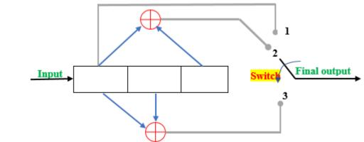
**Q15**. Draw the state diagram, tree diagram and trellis diagram for the L = 3, rate 1/3 code generated by:
